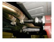
4) Support the rear of the system with a stand. Starting at the rear of the vehicle, remove the three hangers on the right side of the system from the rubber mounts on the vehicle. Unclip the ground strap from the middle hanger on the right tailpipe and using a 15mm socket, loosen the clamps at the slip fit connections behind the catalytic converters. Then with the help of an assistant, lower the stand and slide the system back off of the head pipes. Carefully lower from the vehicle.
